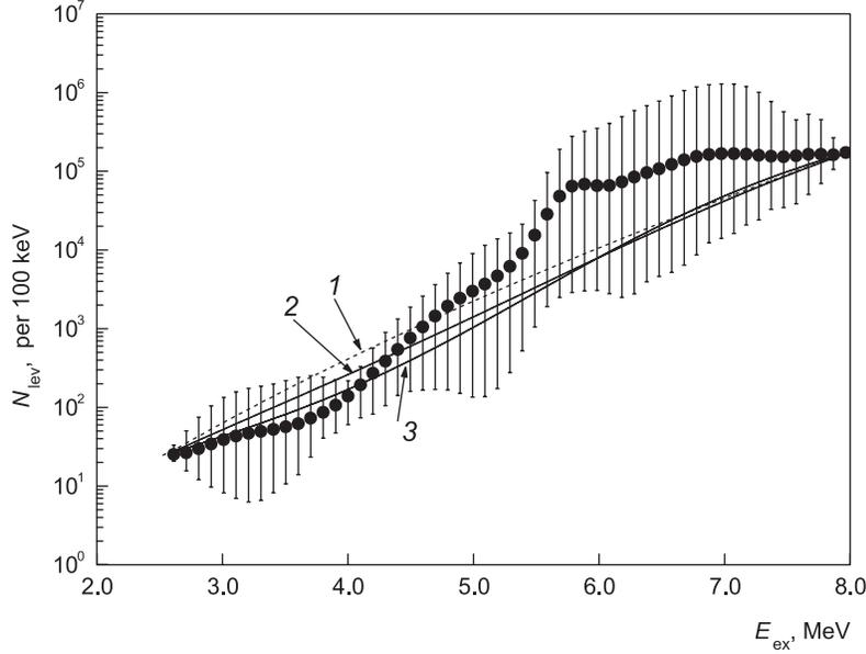
Fig. 2. The interval of variations of the level density providing reproduction of the experimental intensities [8] of the two-step cascades to the ground and first excited state of  $^{172}\text{Yb}$  (points with bars). Line 1 represents predictions according model [14], lines 2 and 3 show the data used in calculations for Figs. 4 and 5, respectively
