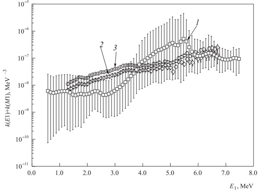
Fig. 3. Interval of variations of the strength functions (points 1 with bars). Points 2 and 3 represent strength functions from [6] and [8], respectively
