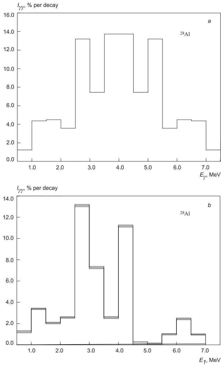
Fig. 1. *a* — the experimental spectrum of the two-step  $\gamma$  cascades terminating at the first and ground states of  $^{28}\text{Al}$ . *b* — distribution [9] of the same intensity in function of the primary transition energy only
